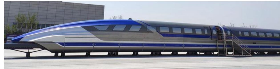
Mockup is pushed on railroad wheels, but only inside the Factory premises because UIC profile exceeded
