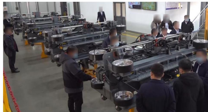
4 suspension frames for the 2-section vehicle
