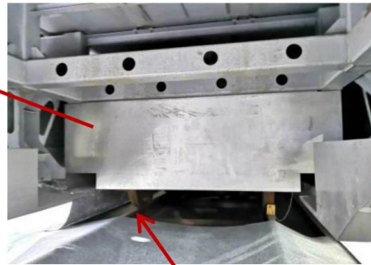
Mockup is pushed on railroad wheels, but only inside the Factory premises because UIC profile exceeded
