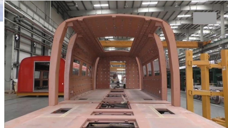
M1 car body: The almost identical construction to the TR08 car body recognizable.
