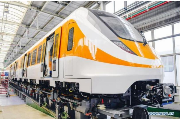
July 6, 2018: Award of the contract to CRRC Manufactured by CRRC Changchun Vmax = 120 km/h 8 poles per SG, nominal air gap 8-10 mm
