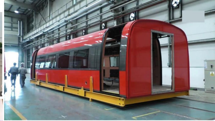
M1 car body: The almost identical construction to the TR08 car body recognizable.
