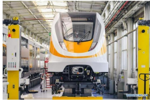
July 6, 2018: Award of the contract to CRRC Manufactured by CRRC Changchun Vmax = 120 km/h 8 poles per SG, nominal air gap 8-10 mm
